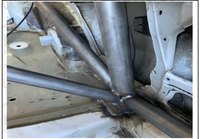
PHOTO 4 MAIN ROLLBAR TO FLOOR ATTACHMENT
