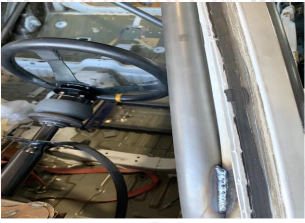
PHOTO 7 FRONT ROLLBAR TO "A" PILLAR ATTACHMENT
