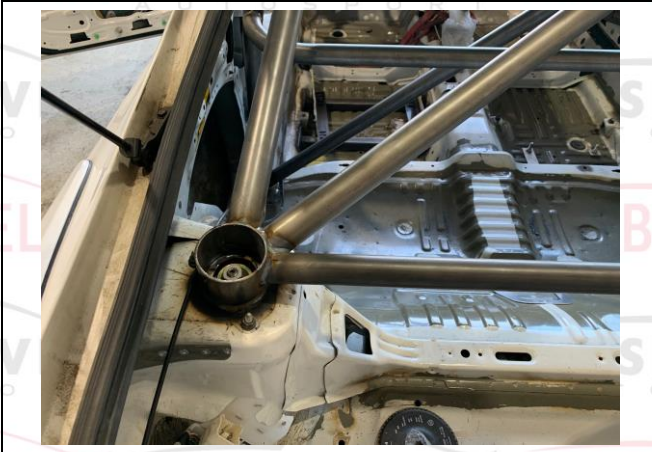
PHOTO 5 REAR BACKSTAY TO BODYSHELL ATTACHMENT
