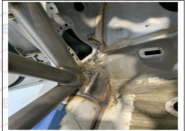
PHOTO 6 FRONT ROLLBAR TO FLOOR ATTACHMENT
