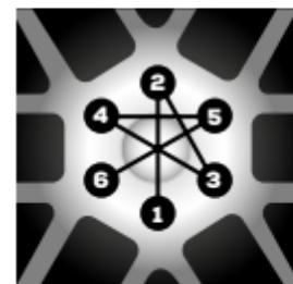
Follow the instructions of the vehicle manufacturer or the rim aftermarket manufacturer to determine the tightening torques of the bolts. It is advisable to carry out static and dynamic checks to ensure that the bolts are correctly tightened. Check the details in the spacer instructions.
